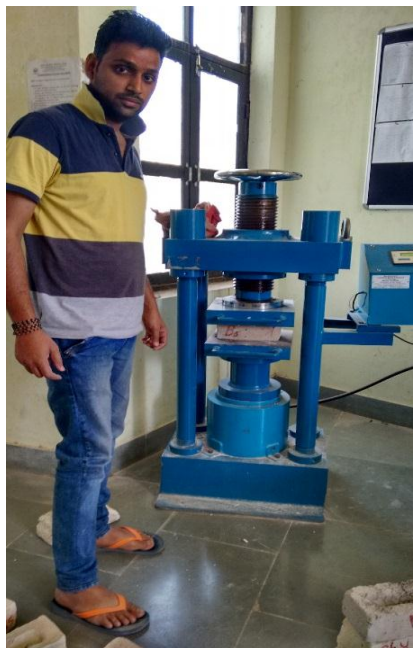
Figure 2: Setup of Compression Strength Test
