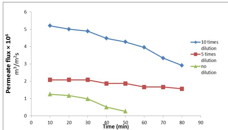
Fig. 4: Permeate flux v/s time for EG-water feed at  $5 \text{ kg/cm}^2$
