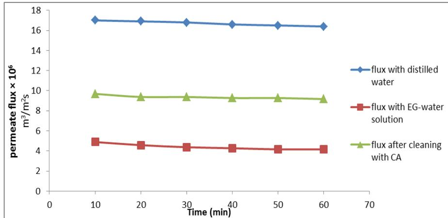
Fig. 5: Permeate flux v/s time for chemical cleaning with citric acid at 5 Kg/cm<sup>2</sup>
