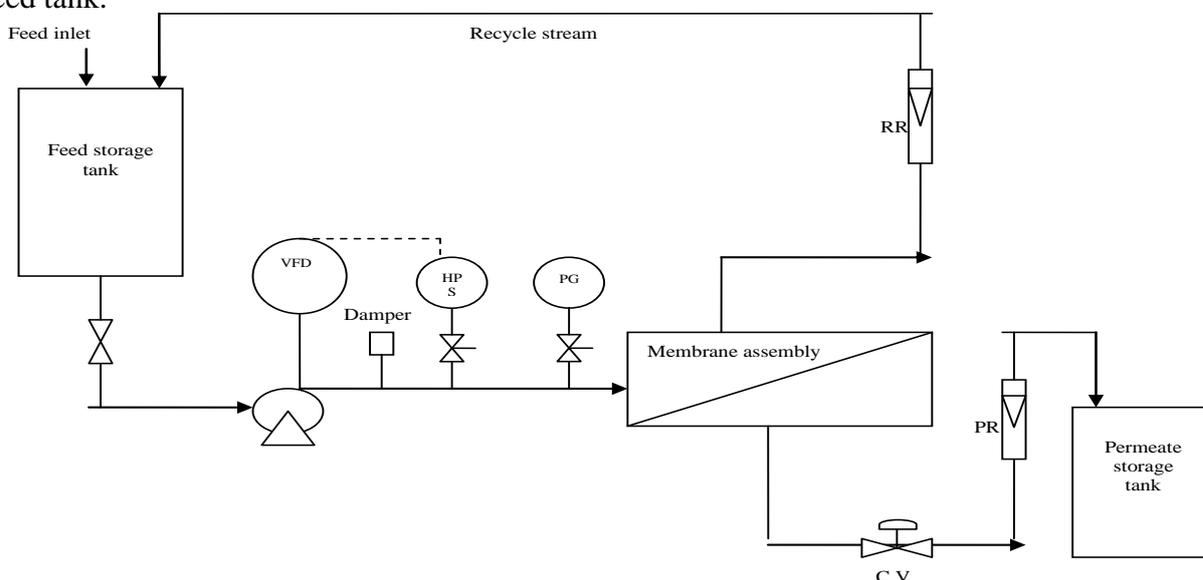
Fig. 1: Schematic of experimental setup for nanofiltration
