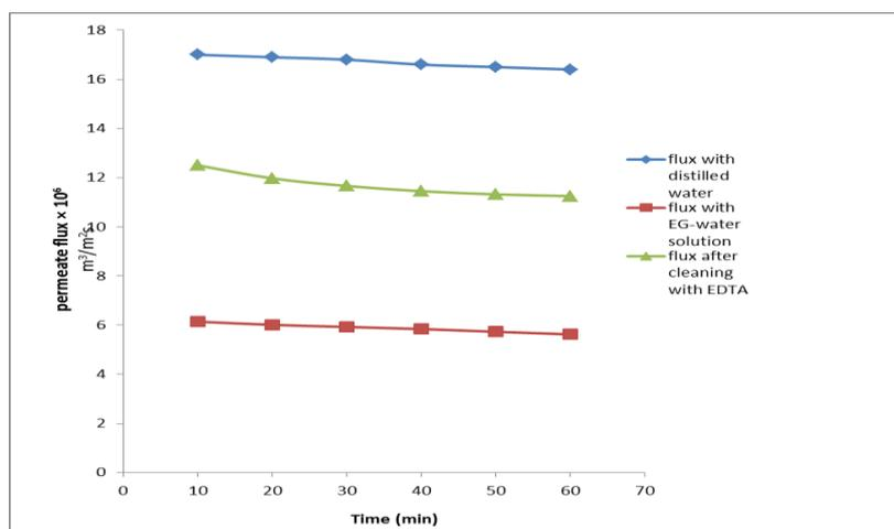
Fig. 6: Permeate flux v/s time for chemical cleaning with EDTA at 5 Kg/cm<sup>2</sup>
