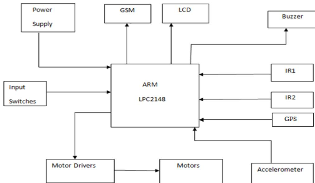
Figure 1. Block diagram
