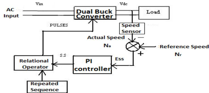
Fig: 1 Block Diagram of closed loop control four quadrant DC-Drive
