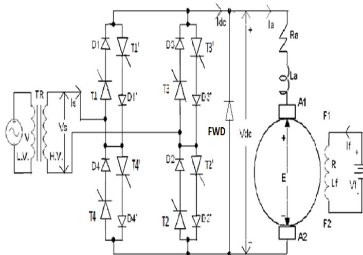
*Fig:2 Conventional single-phase, dual ac-dc buck converter fed four-quadrant, armature controlled, separately excited dc drive*
