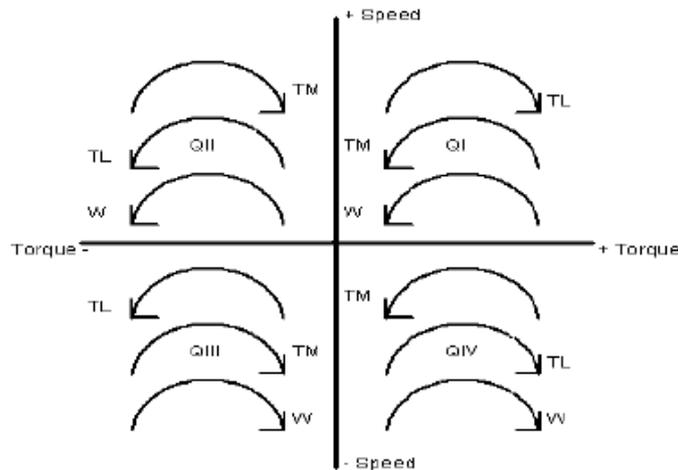
Fig. 3.3. Speed-torque plane with the four quadrants demarcated
