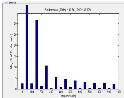
Fig 9.0 FFT of ac side current for quadrant I operation
