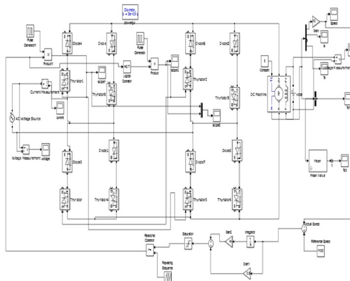
Fig: 4. Closed loop Block Diagram implementation of four quadrant fed DC drive
