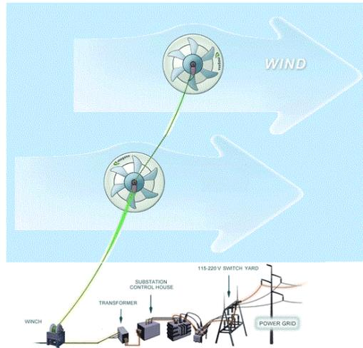
**Figure 4: Ladder Mill Connected To Grid**
