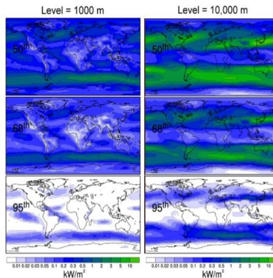
Figure 7: Wind power density ( $\text{kW}/\text{m}^2$ ) that was exceeded 50%, 68%, and 95% of the time during 1979-2006 at 1,000 m (left) and 10,000 m (right) from the NCEP/DOE re analyses<sup>[2][5]</sup>.
