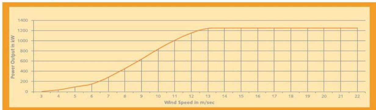
Figure 9: Power Output With Respect To Wind Speed.
