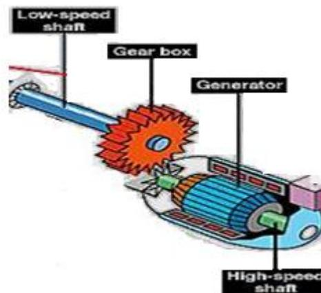
Figure 3: Shafts, Gear Box and Generator
