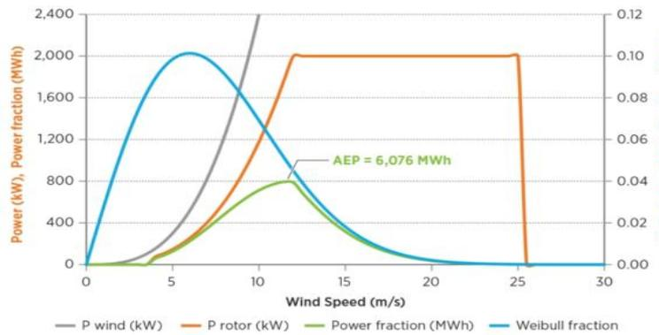
**Figure 10: Variation of Various Parameters with wind speed**
