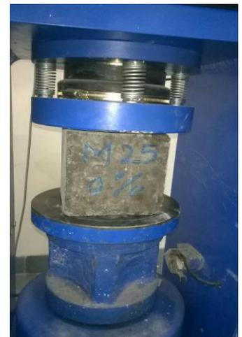
“Figur3. Compressive Strength Test set up”
