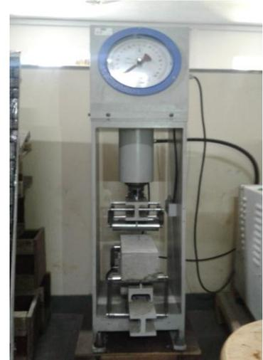
“Figure4 .flexural Strength Test set up”
