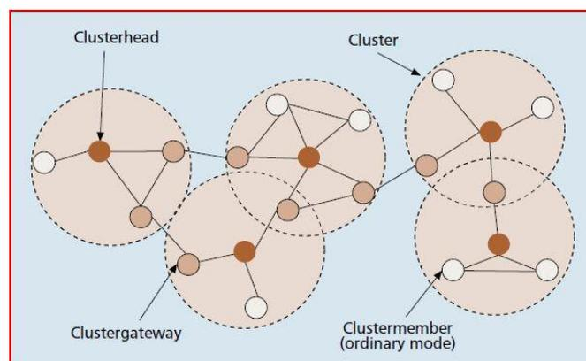
Fig 1: Structure of nodes
