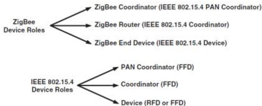
Fig. 3. Device Roles in the IEEE 802.15.4 and ZigBee Standards
