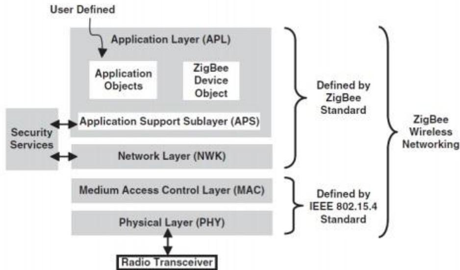
Fig. 2. ZigBee Wireless Networking Protocol Layers
