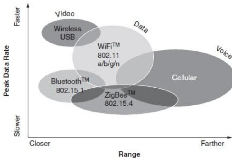
Fig. 1. Wireless Technologies Compared
