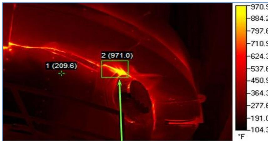
*Fig.5. Gas leaks in thermal image*
