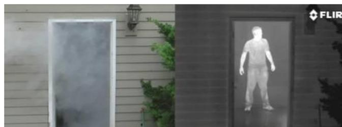
*Fig. 12 Thermal Image in smoke*
