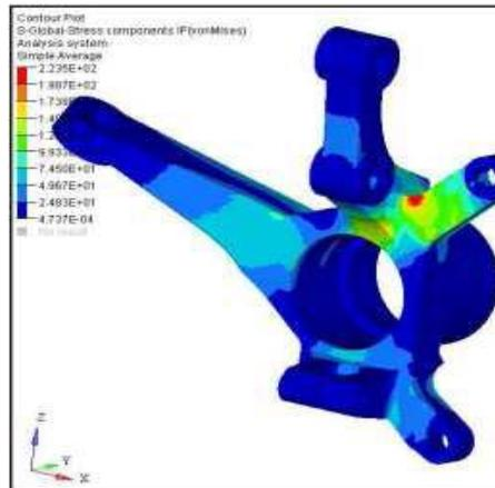
Fig.3. Stress in KNUCKLE JOINT[2]
